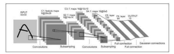
Figure 4: The Structure of the LeNet Neural Network.
